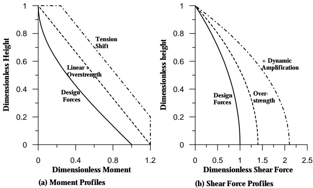
**Fig.1 Dynamic Amplification of Design Forces for Equivalent Lateral Force Design Of Cantilever Walls.**
