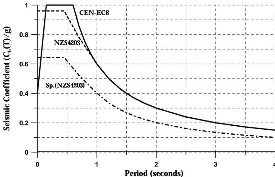
**Fig.2 Comparison of EC8 spectrum for 0.4g PGA with NZS4203 for Z = 1.2**
