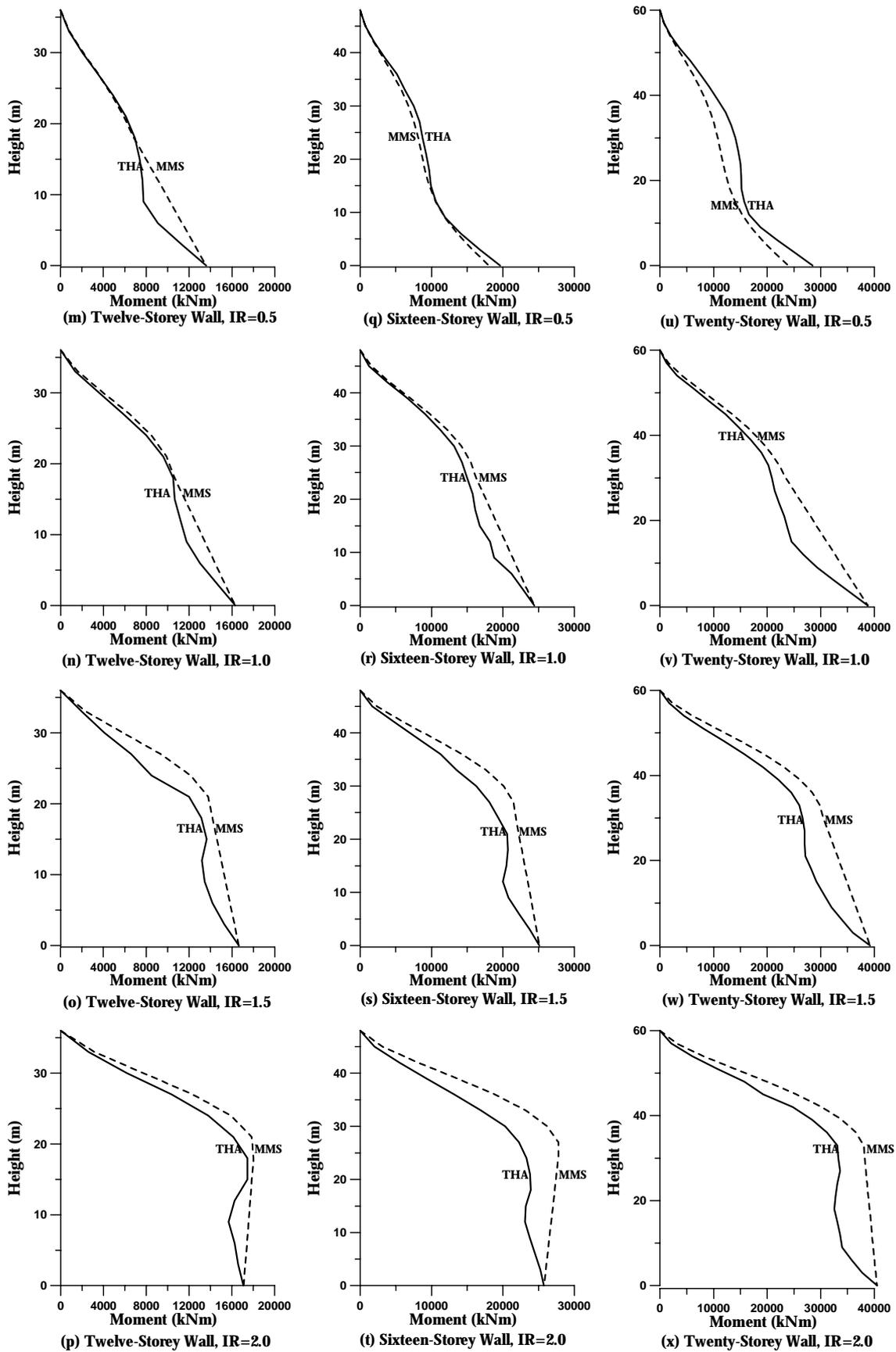
**Fig.8 (cont). Comparison of Modified Modal Superposition (MMS) Moment Envelopes With Results from Inelastic Time-History Analysis for Different Seismic Intensities**
