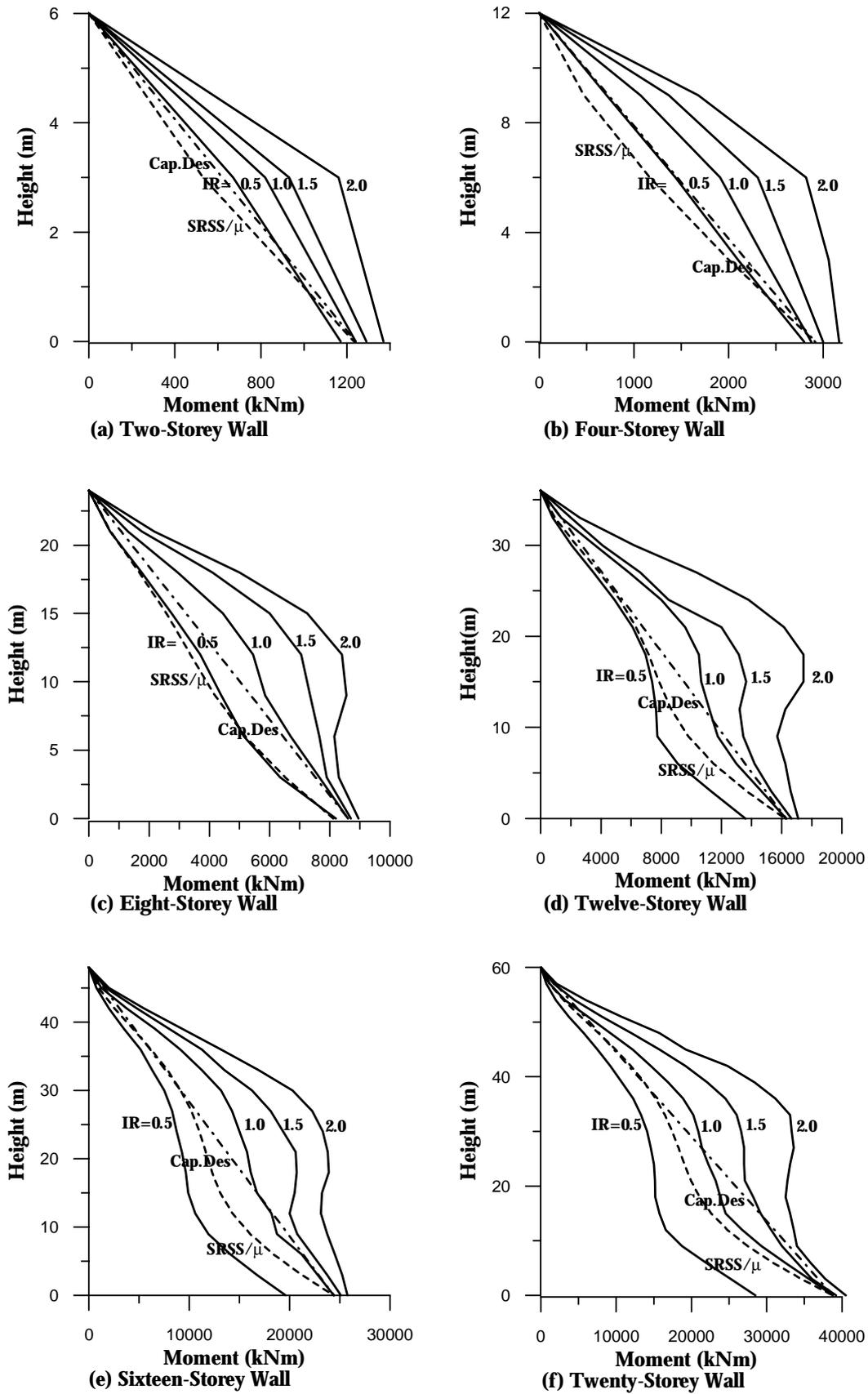
**Fig.6 Comparison of Capacity Design Moment Envelopes with Results of Time-History Analyses For Different Seismic Intensity Ratios**
