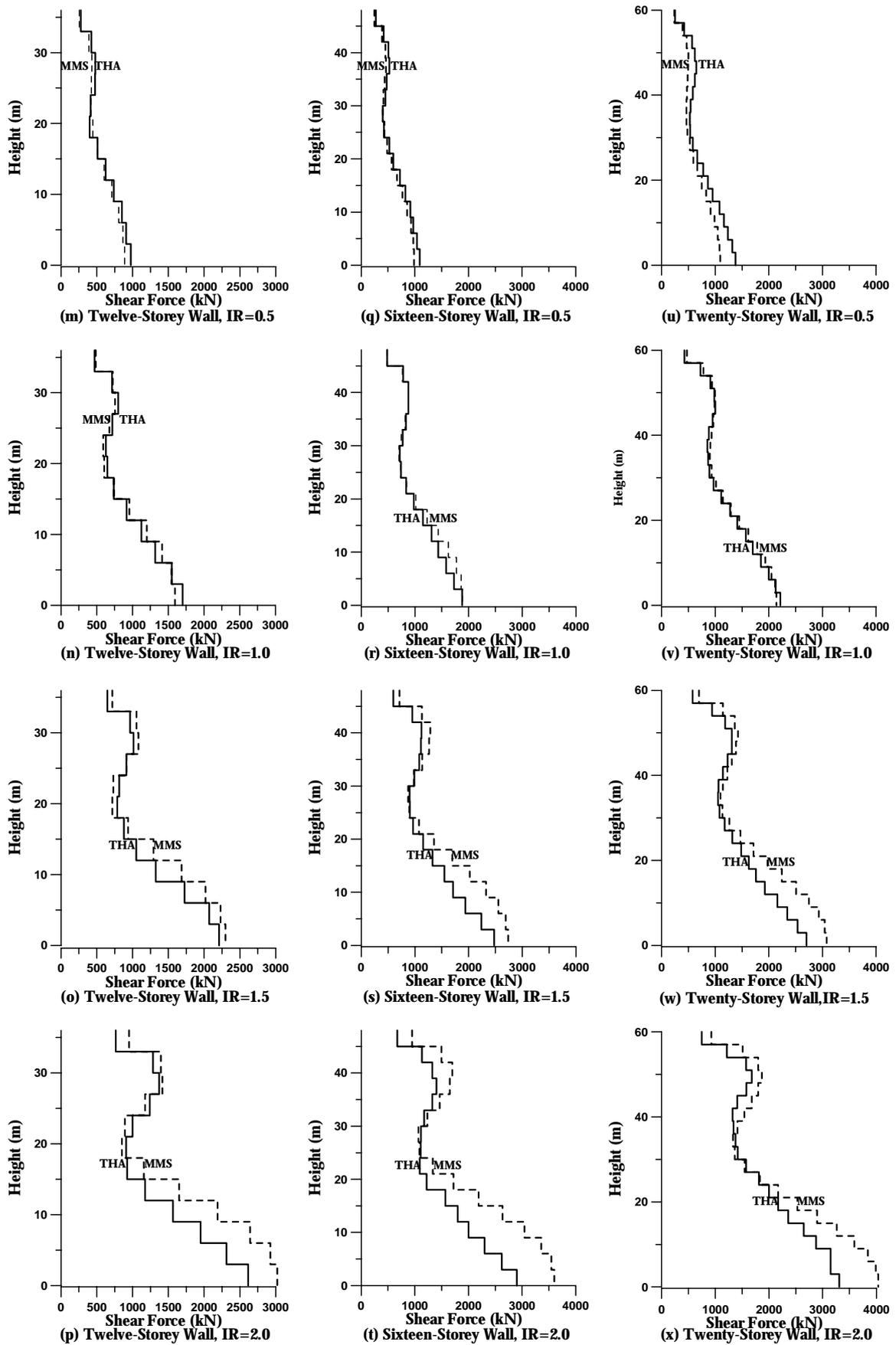
**Fig.9 (cont) Comparison of Modified Modal Superposition (MMS) Shear Force Envelopes With Results from Inelastic Time-History Analysis, for Different Seismic Intensities**
