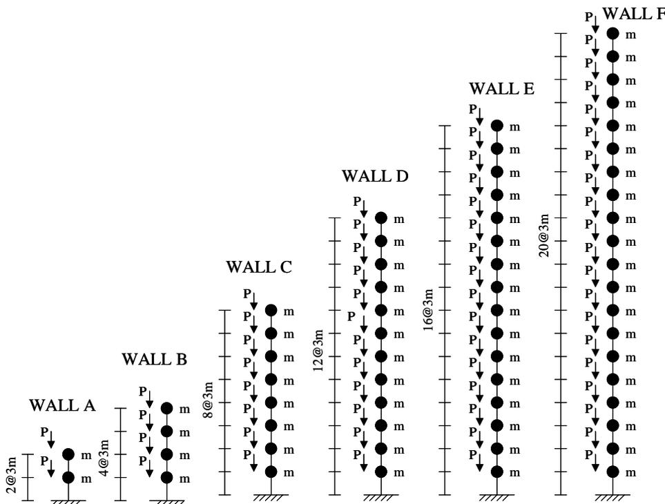
**Fig.3 Idealization of Cantilever Walls**
