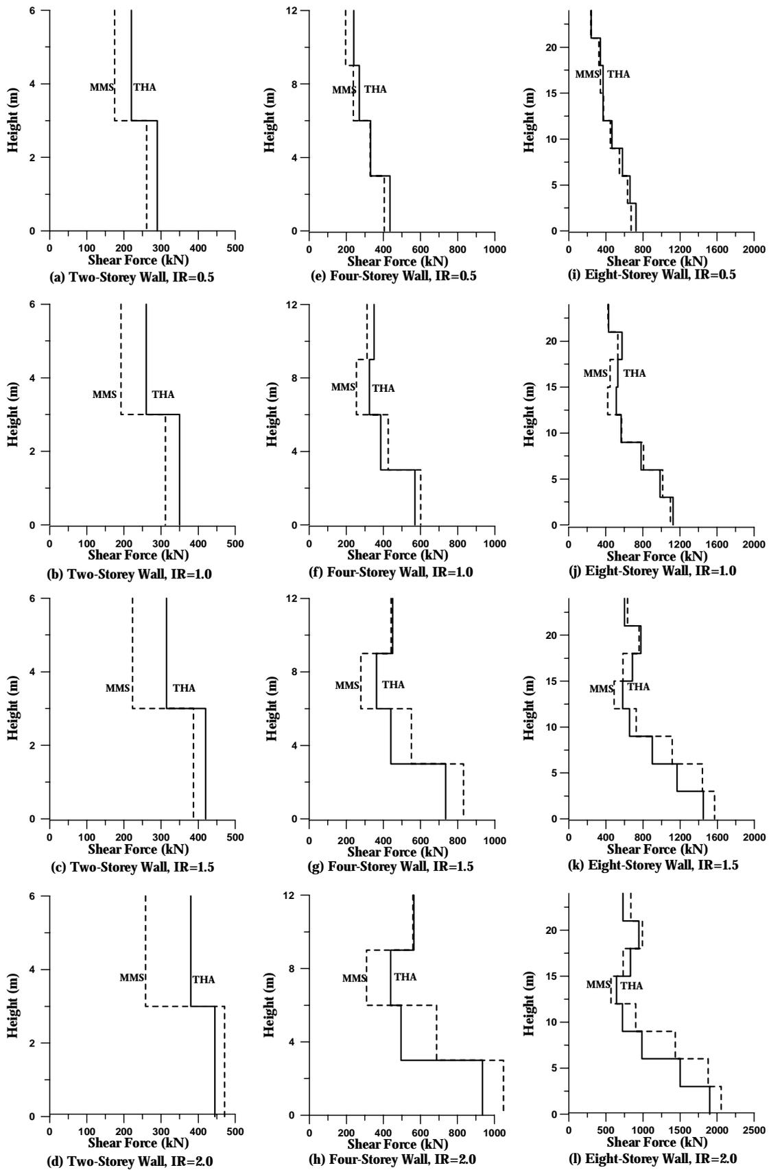
**Fig.9 Comparison of Modified Modal Superposition (MMS) Shear Force Envelopes With Results from Time-History Analyses for Different Seismic Intensities**
