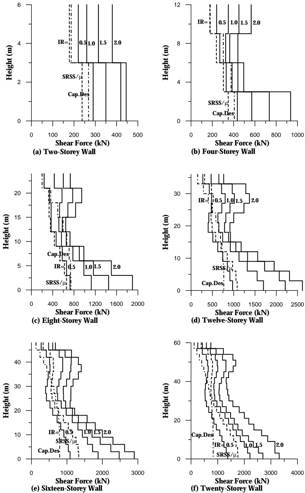
**Fig.7 Comparison of Capacity Design Shear Force Envelopes with Results of Time-History Analyses for Different Seismic Intensity Ratios**
