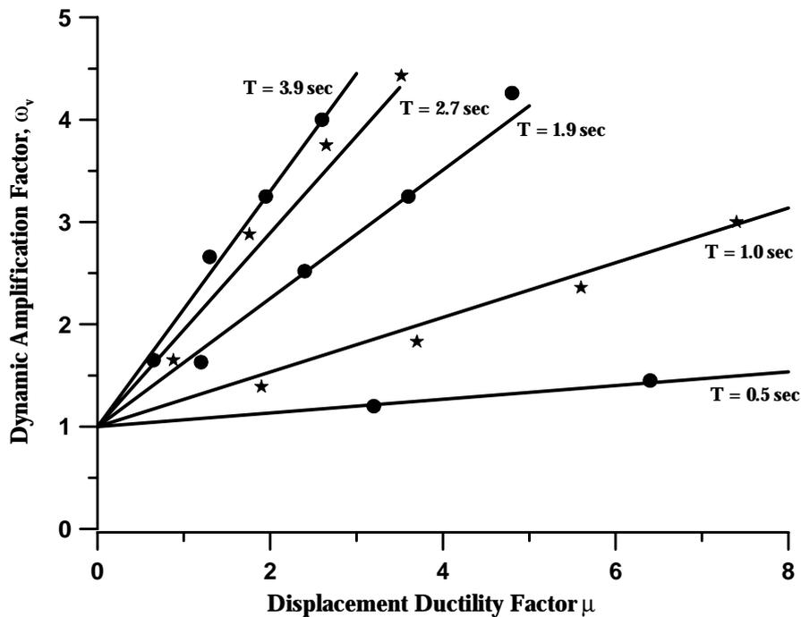
**Fig.10 Wall Base Shear Force Dynamic Amplification Related to Period and Ductility (data points from time-history analyses; lines from Eq.(10))**
