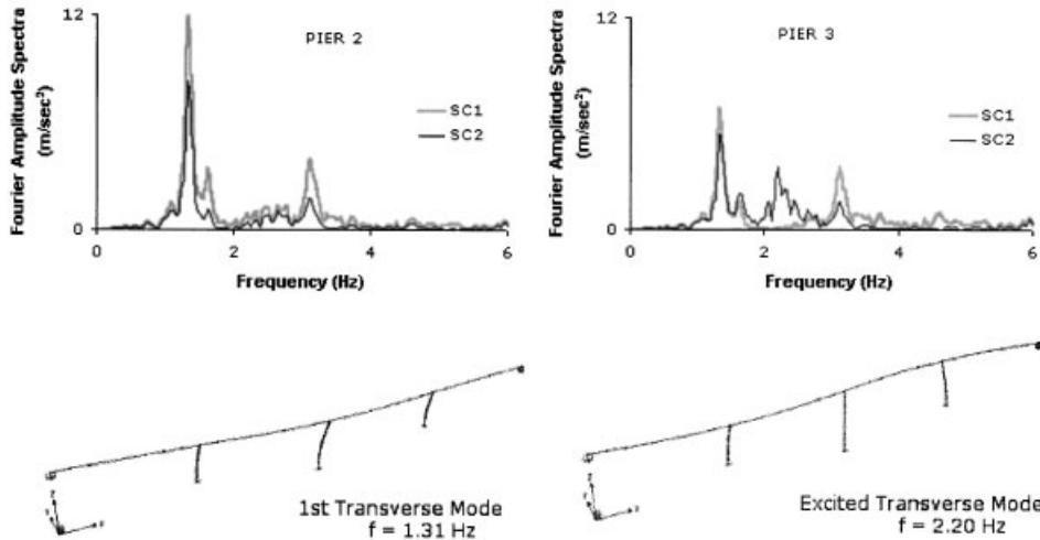
Figure 7. Fourier amplitude spectra of Pier 2 (model C3) for wave passage effect (SC2) and 'standard' approach (SC1).
