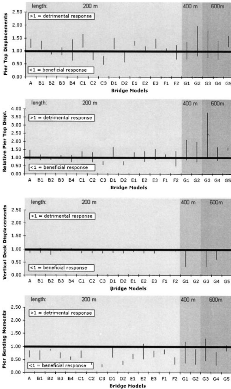
Figure 12. SSI (SC6) response parameters normalized to non-SSI case (SC4).
