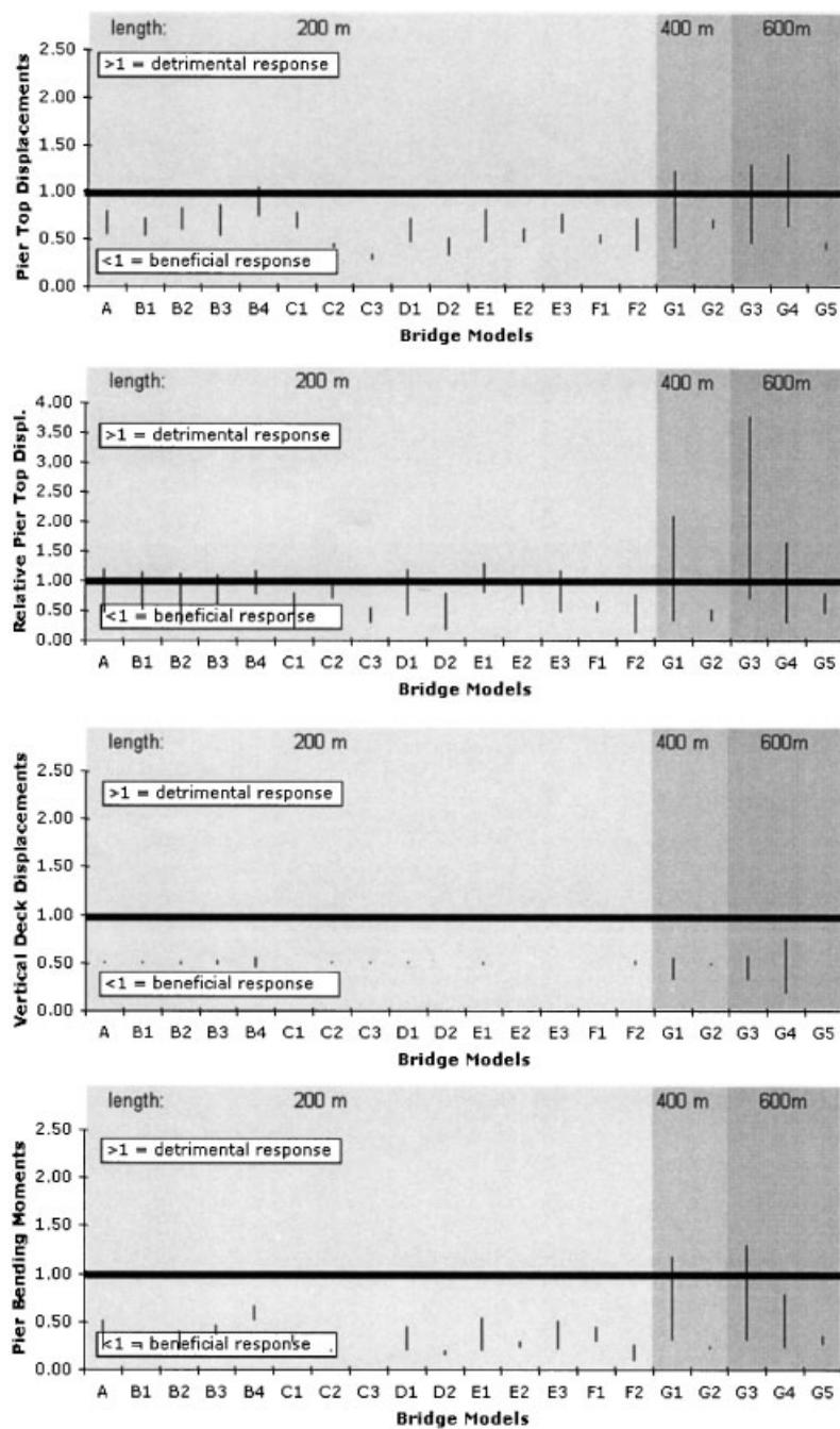
Figure 13. SSI, uniform excitation (SC7) response parameters normalized to 'standard' approach (SC1).
