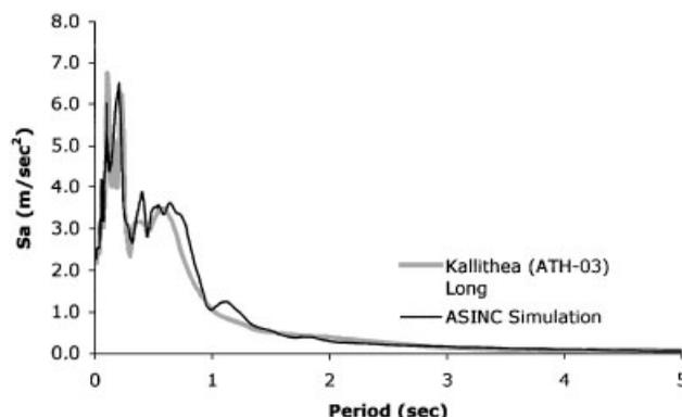
Figure 2. Comparison between target and simulated motion acceleration response spectrum.
