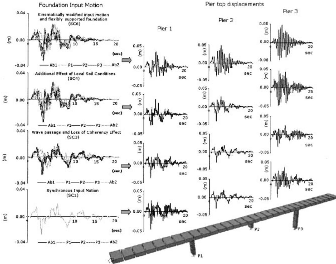
Figure 5. Pier top transverse response under various excitation scenarios.
