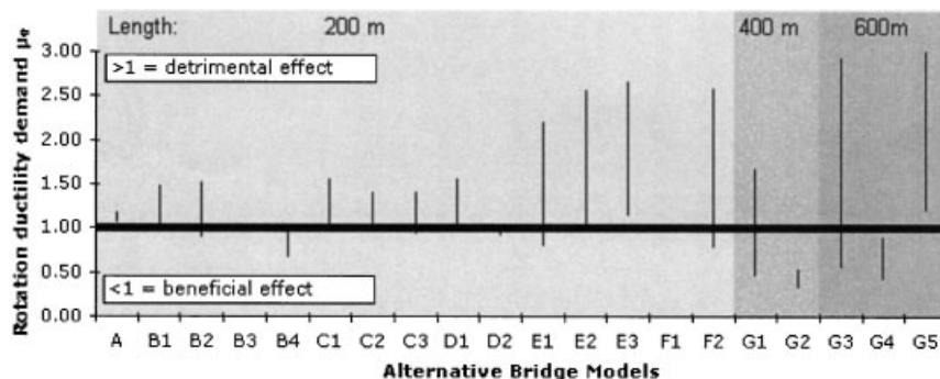
Figure 14. ‘Complete’ inelastic analysis (SC8) ductility demand normalized to ‘standard’ inelastic analysis approach (SC9).
