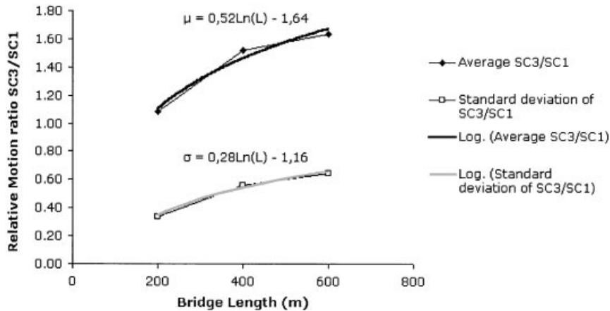
Figure 10. Relative motion dependency on overall bridge length.
