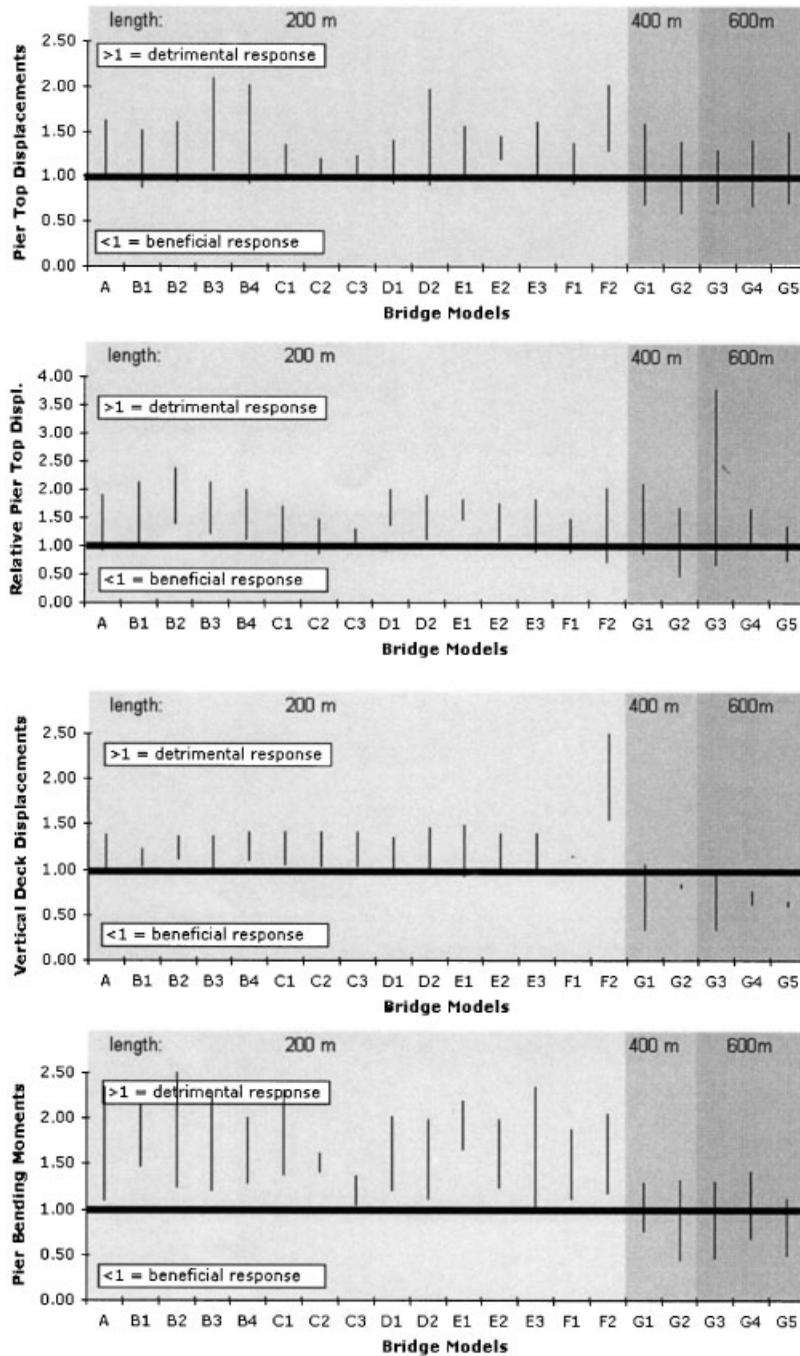
Figure 11. Site Effects (SC4) response parameters normalized to non-site effects case (SC3).
