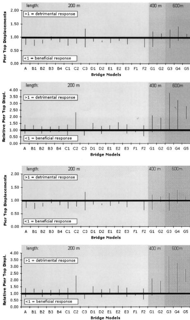
Figure 6. Wave passage effect (SC2) response parameters normalized to 'standard' approach (SC1).
