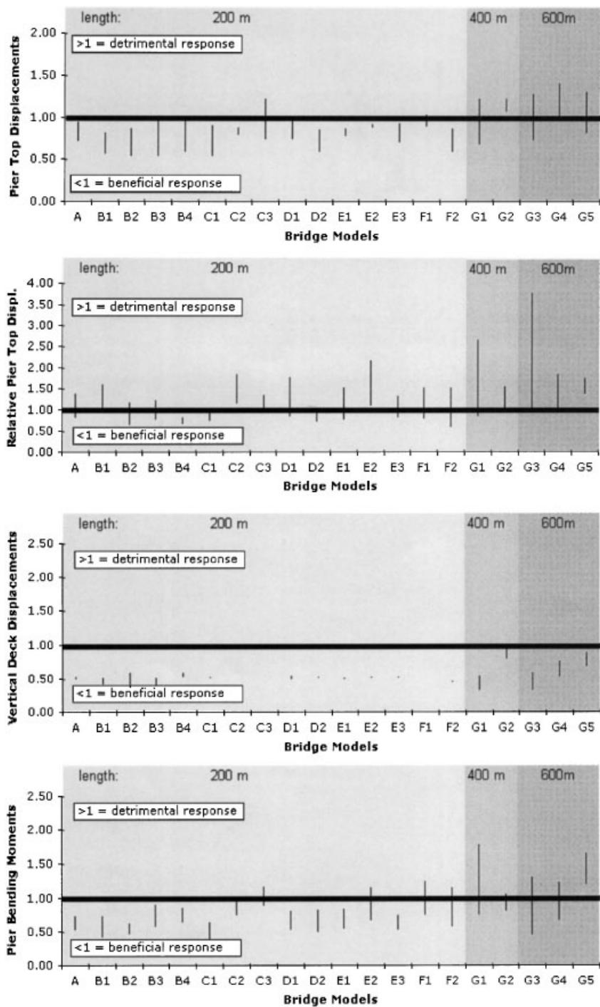
Figure 8. Loss of coherency (SC3) response parameters normalized to 'standard' approach (SC1).
