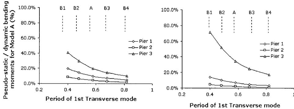
Figure 9. Pseudostatic force increase with structural stiffness for excitation that accounts (a) for the wave passage effect (b) for wave passage effect and loss of coherency.
