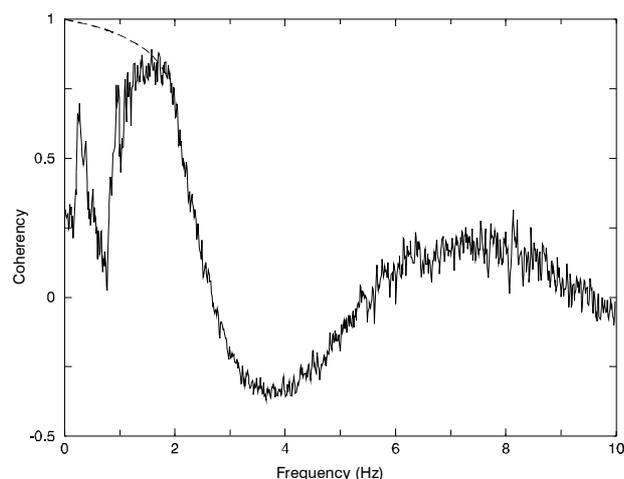
Fig. 8. Azimuthally-averaged coherencies for the BHP site, using triangular arrays with 15m sides. Dashed line shows the expected form of coherency if Rayleigh waves dominate the microtremors.
