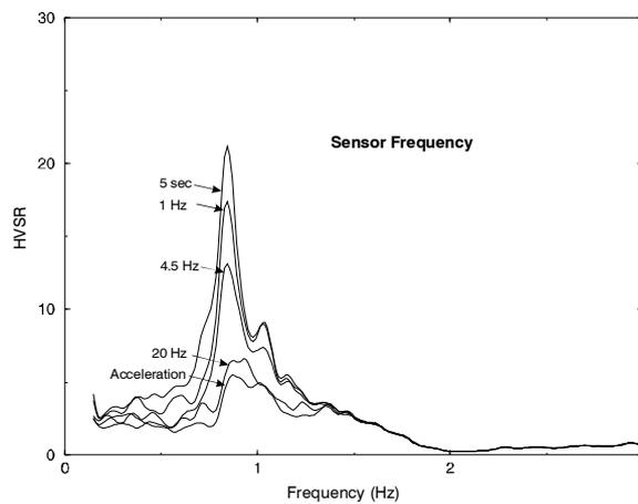
Fig.3. Horizontal-to-vertical spectral ratios at the BHP site for various sensors. A 4-bit digitizer is assumed, together with gain-ranging using 16 $\times$  steps.
