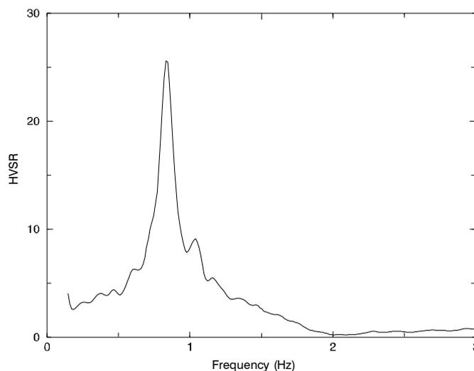
Fig. 2. Horizontal-to-vertical spectral ratio at the BHP site using original data. This curve corresponds to all cases for which high frequency geophones have been simulated, provided that low-noise, gain-ranging digitizers with 8-bit or over resolution, are used.
