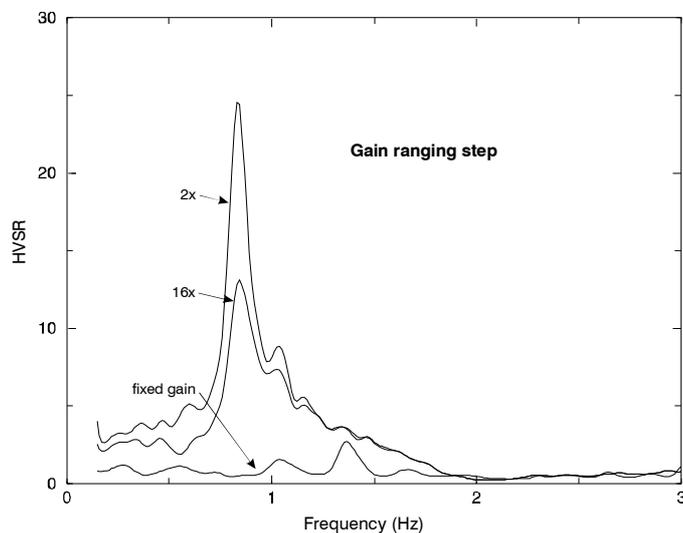
Fig 5. Horizontal-to-vertical spectral ratios at the BHP site for various gain ranging steps. A 4.5 Hz geophone is assumed, together with a 4-bit digitizer resolution.
