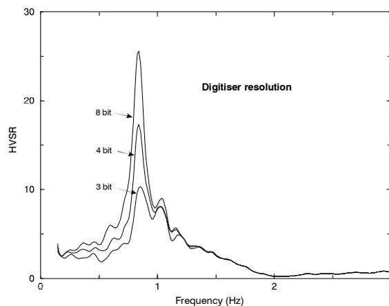
Fig 4. Horizontal-to-vertical spectral ratios at the BHP site for various digitizer resolutions. A 20 Hz geophone is assumed, together with gain-ranging using 2 $\times$  steps.
