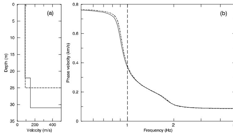
Fig. 6. (a) Alternative shear wave profiles assumed for the BHP site. (b) Dispersion curves corresponding to the profiles of (a). Dashed vertical line marks the frequency below which Rayleigh waves are thought to cease dominating.
