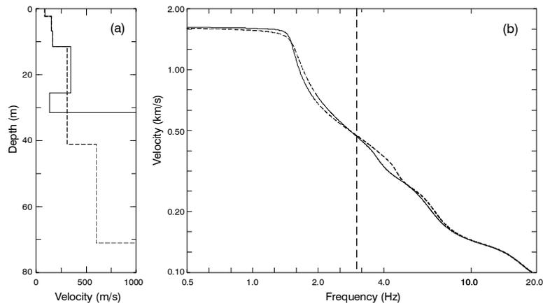
Fig. 7. (a) Alternative shear wave profiles assumed for the PKW site. (b) Dispersion curves corresponding to the profiles of (a). Dashed vertical line marks the frequency below which Rayleigh waves are thought to cease dominating.
