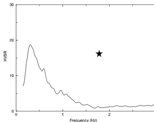
Fig. 9. Horizontal-to-vertical spectral ratio at the MCE site. Asterisk marks the frequency at which a peak is to be expected on the basis of resonance of the top, 21 m thick, soil layer.
