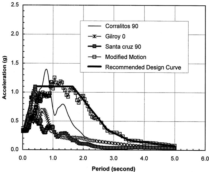
FIGURE 35.11 Acceleration response spectra for Sonoma Creek Bridge.
