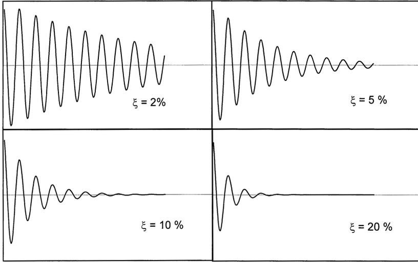
FIGURE 35.6 Response of an SDOF system for various damping ratios.
