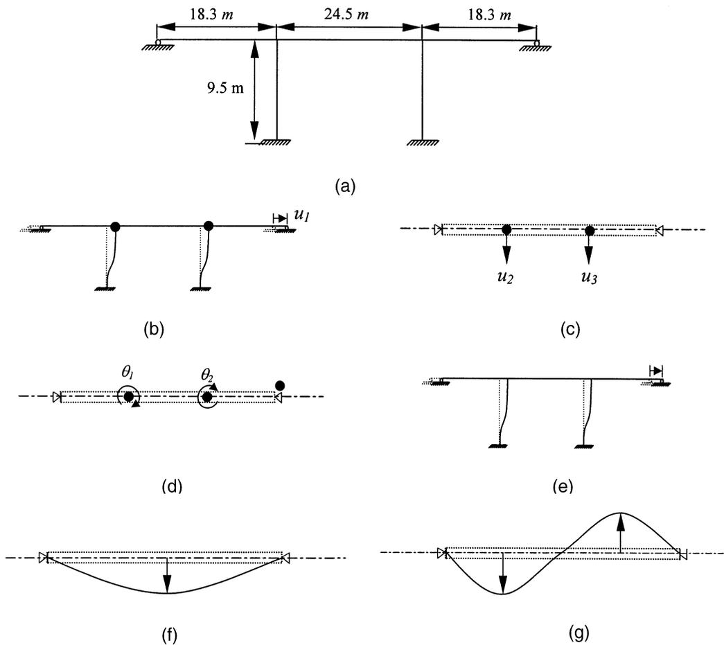
**FIGURE 35.16** Three-span continuous framed bridge structure of MDOF example. (a) Schematic diagram; (b) longitudinal degree of freedom; (c) transverse degree of freedom; (d) rotational degree of freedom; (e) mode shape 1; (f) mode shape 2; (g) mode shape 3.
