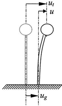
FIGURE 35.4 Earthquake-induced motion of an SDOF system.
