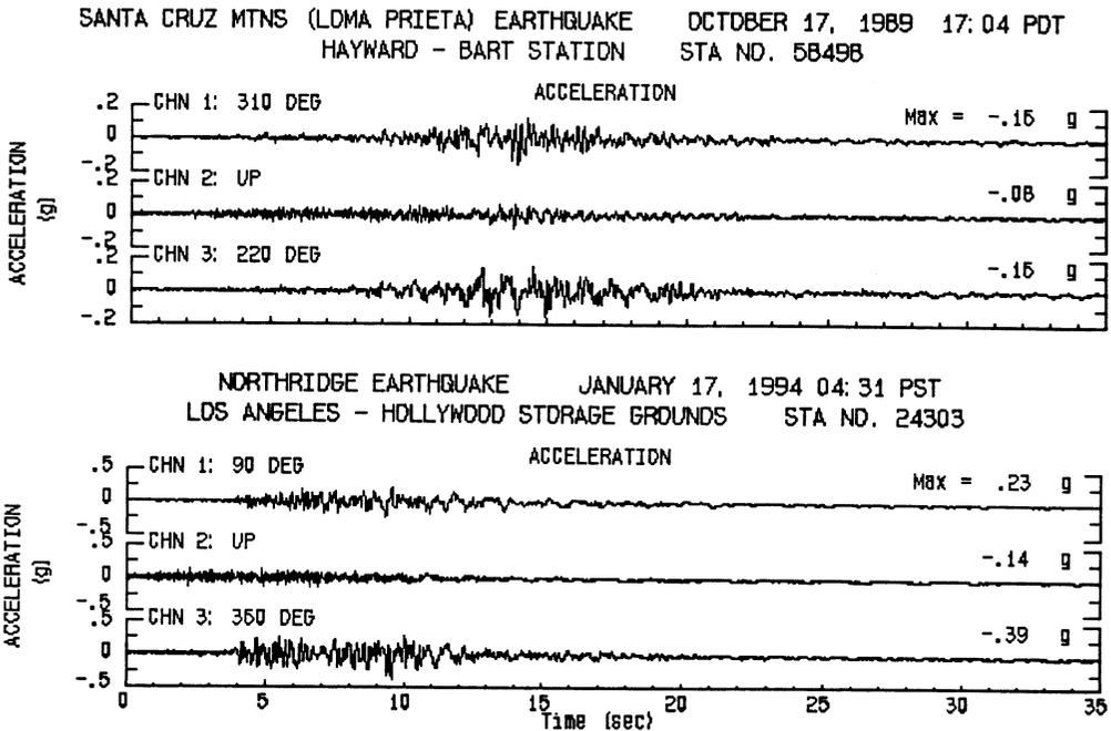
FIGURE 35.1 Ground motions recorded during recent earthquakes.
