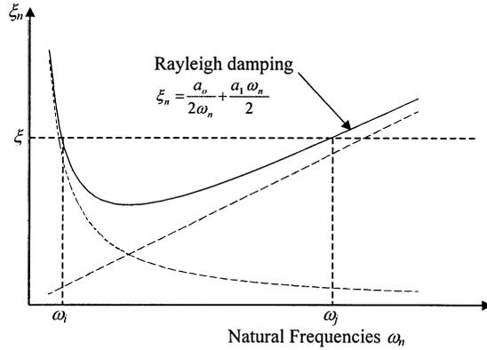
FIGURE 35.15 Rayleigh damping variation with natural frequency.
