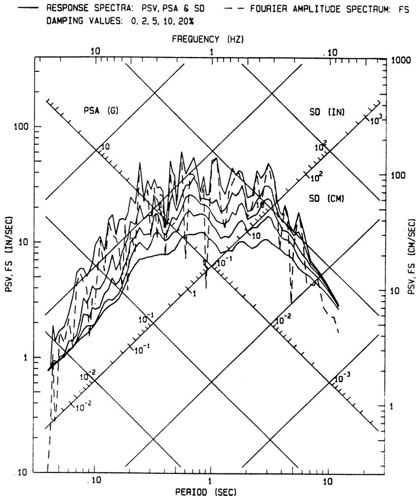
FIGURE 35.9 Tripartite plot—response spectra (1994 Northridge Earthquake, Arleta–Rordhoff Ave. Fire Station).
