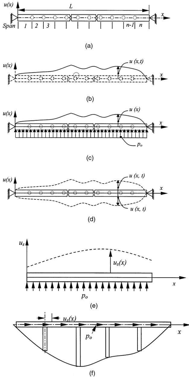
**FIGURE 35.18** Single-mode spectral analysis method. (a) Plan view of a bridge subjected to transverse earthquake motion. (b) Displacement function describing the transverse position of the bridge deck. (c) Deflected shape due to uniform static loading. (d) Transverse free vibration of the bridge in assumed mode shape. (e) Transverse loading (f) longitudinal loading.
