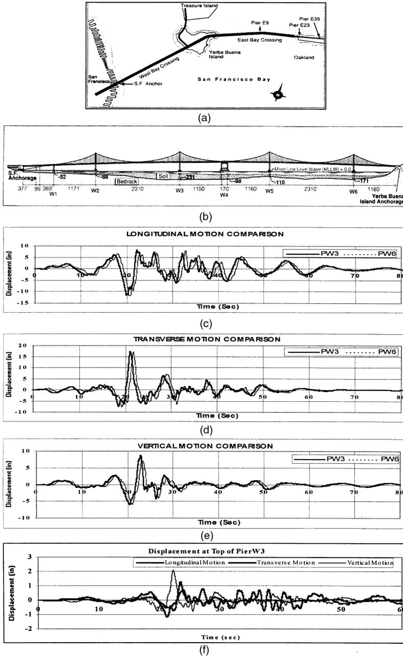
FIGURE 35.17 San Francisco–Oakland Bay Bridge. (a) Vicinity map; (b) general plan elevation; (c) longitudinal motion at rock level; (d) transverse motion at rock level; (e) vertical motion at rock level; (f) displacement response at top of Pier W3.
