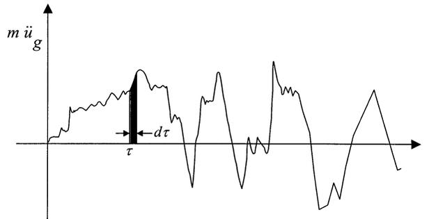
FIGURE 35.7 Induced earthquake force vs. time on an SDOF system.
