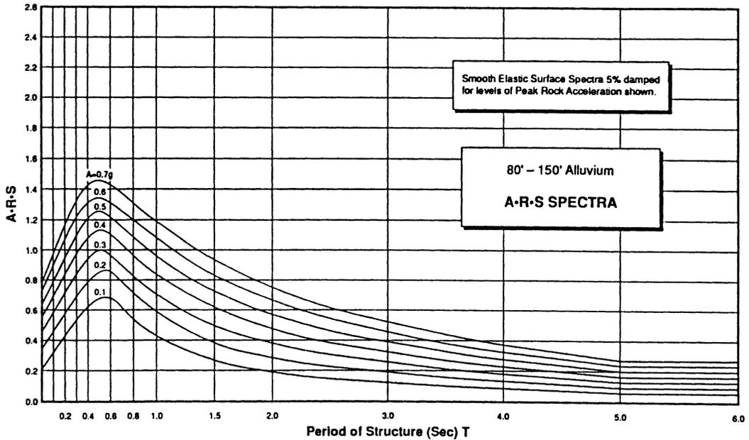
FIGURE 35.10 Typical Caltrans elastic design response spectra.
