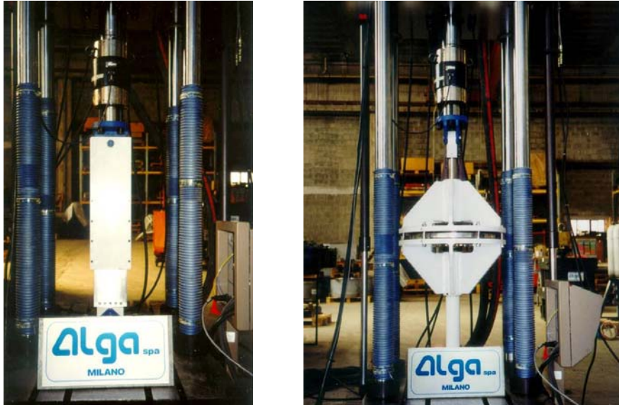
Fig. 6.8. ER Dampers: linear (left) and rotating (right) working schemes (Marioni, 2002)
