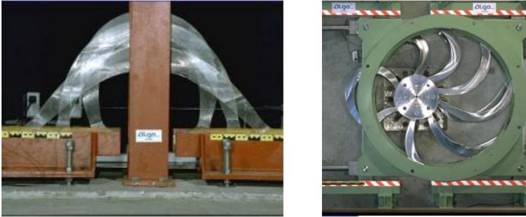
Fig. 3.13. C-shaped device (left) and EDU device (right)
