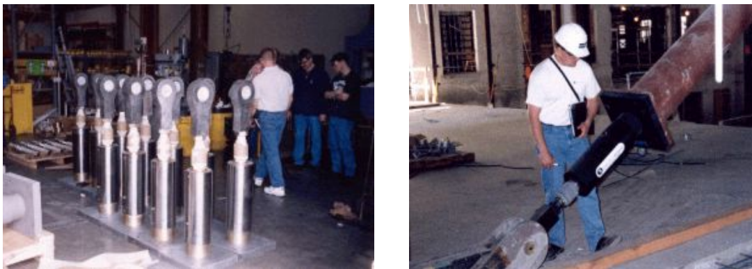
Fig. 4.7. The Taylor device: San Francisco Civic Center dampers
