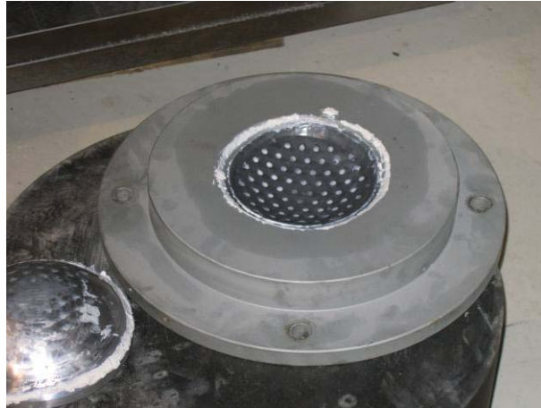
Figure 2 Base plate of the single surface sliding pendulum
